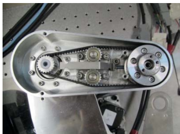
Fig2. Belt and pulley in arm
