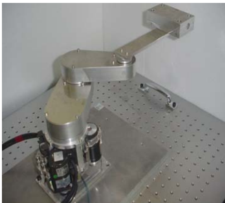
Fig1. Belt driving robot
